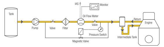
Float or valve control in the intermediate tank is required. Formation of gas is to be avoided. The magnetic valve opens as soon as the pressure drops below a defined level. For measuring the consumption of more than one engine, each will require a separate installation similar to the one above.
