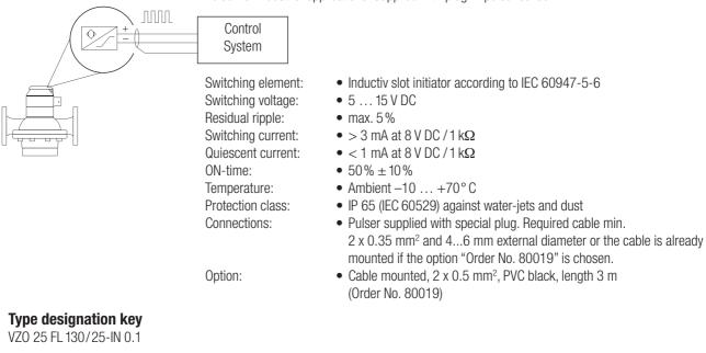
Pulser IN or RV and pulse value Nominal pressure bar Temperature °C Connection (RC = Threaded ends, FL = Flanges) Dimension mm Type
