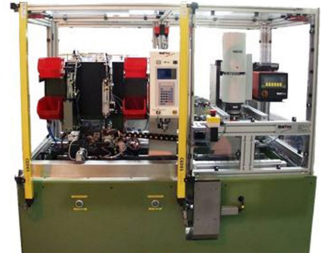
Oil pump assembly station to assemble the over pressure valve. This includes a test of the spring compression force, a cup plug electro-press and a radial riveter to secure the cup in place
