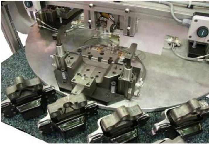
Rotary assembly station to clamp a gearbox vibration mount together before riveting
