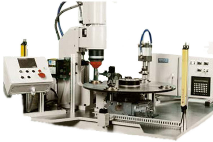
Radial forming system with automatic air leak testing – Automotive
