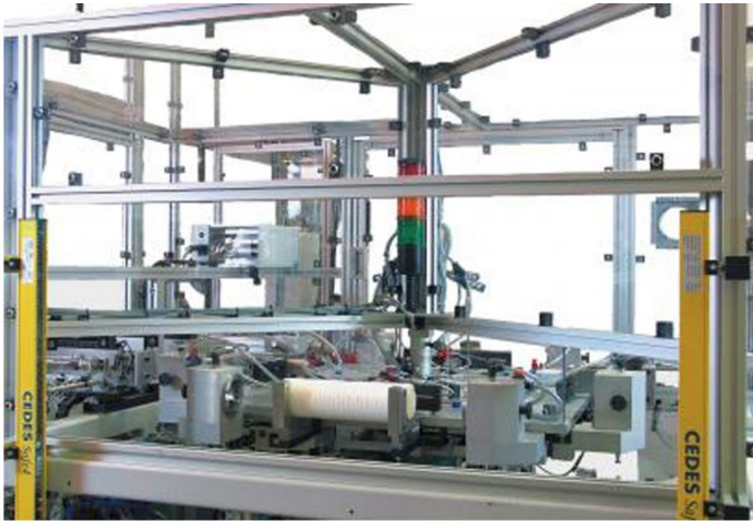
Rotary assembly machine to plastic weld a variation of end caps to medical filter cartridge
