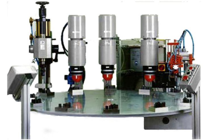
Multi riveting head system with engraving station automatic door lock assembly
