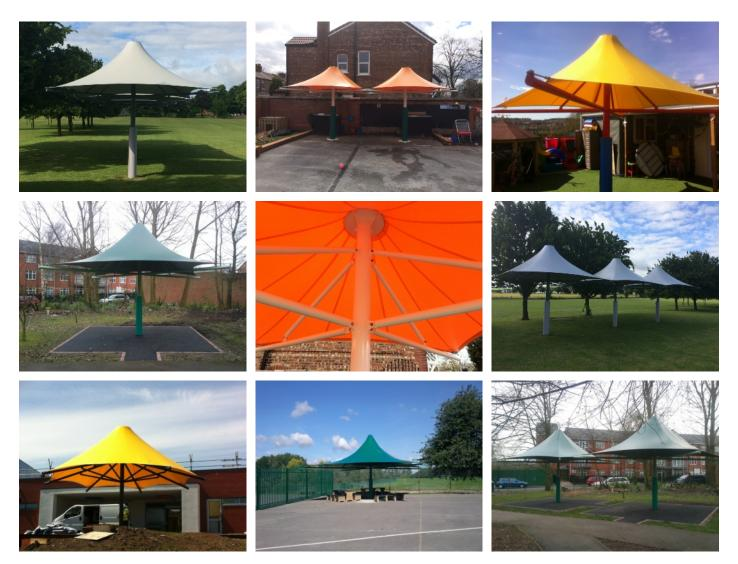
Folding umbrellas offer a low cost, versatile alternative to other types of structure. The structures are available with many different support type options & are complimented by a huge fabric range. The main advantage of folding umbrellas is that they can be folded down & covered when not in use.
