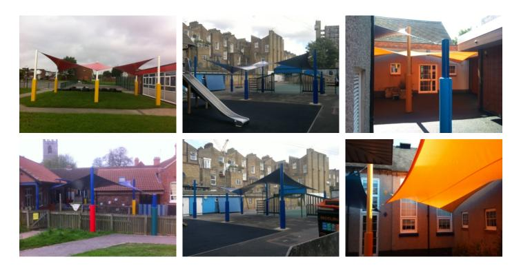
Conical structures are specifically designed to cover a large area with a single fabric canopy. Having multiple perimeter support posts & a single central support post means that we can cover a larger single area than with any other type of structure thus offering many possibilities for continued outdoor use.
