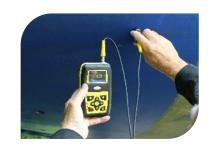
All probes have Intelligent Probe Recognition (IPR), which automatically adjusts settings in the gauge at the same time as transmitting recognition data - the result is a perfectly matched probe and gauge for enhanced performance.
