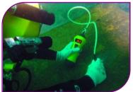
All measurements are error checked to ensure only accurate readings are displayed, even on uncoated metal. The gauge is simple to use, with little operator input, and has a large bright 10 mm display which ensures it can be easily read by the diver, even in poor visibility. It easily upgrades to a topside repeater with either a surface display unit or datalogging option.
