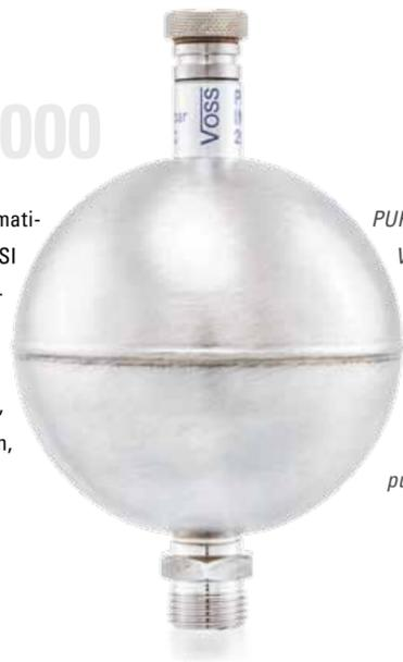
*PURG-INOX 2.000 Automatic Float Air Vent are made of AISI 316Ti Stainless Steel for use under extreme conditions up to 16 bars, where high material resistance is indispensable as in district heating plants, water plants, water conditioning plants, pumps, industrial applications, etc.*
