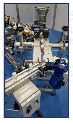
Automatic filling and cap tightening
