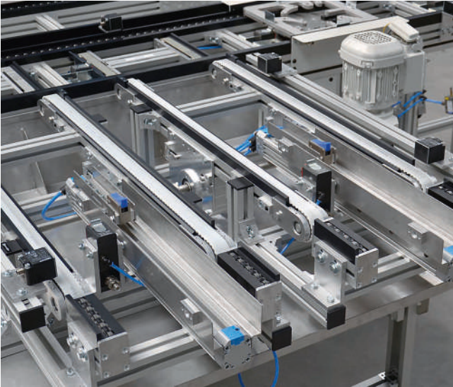
Lift and transfer with component monitoring and end position sensor
