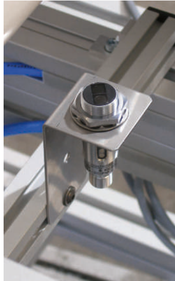
Initiator holder made from VA steel sheet
