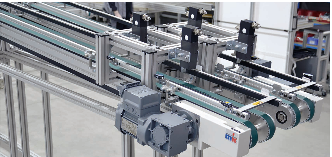
Double dual-line timing belt conveyor ZRF-P 2040 with separation unit and adjustable incline
