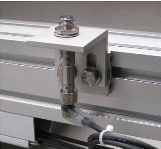
Initiator holder made from aluminium angle bracket
