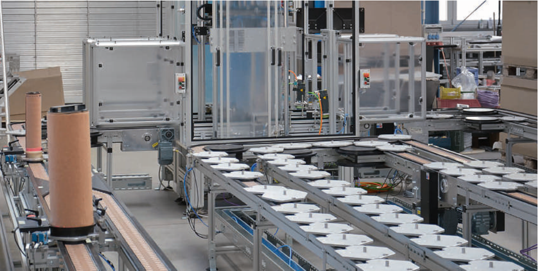
Automated interlink with pallets, including rotating, stopping, separating and centring, based on flat top chain conveyor
