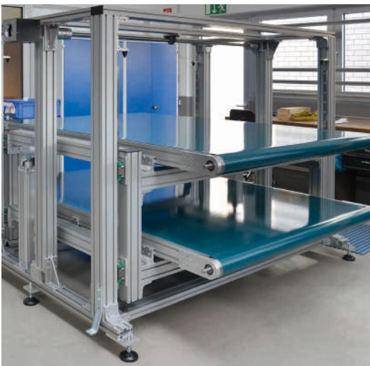
C-frame with recirculating ball bearing guides, each with 2 roller carriages for lifting or lowering the GUF-P 2004 conveyors
