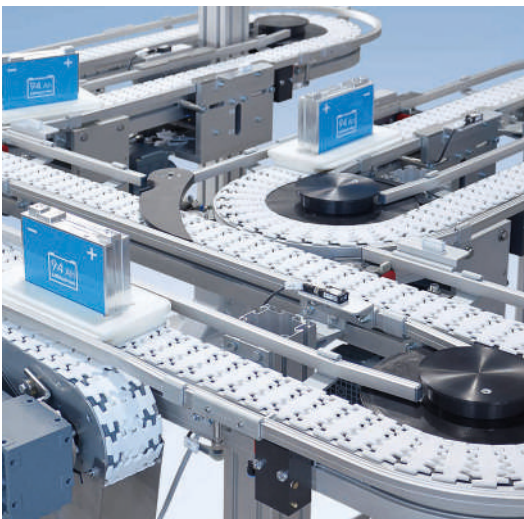
SBF-P 2254 with transfer pusher for the packaging industry, for instance
