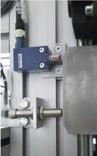
Sensors for deceleration and stopping
