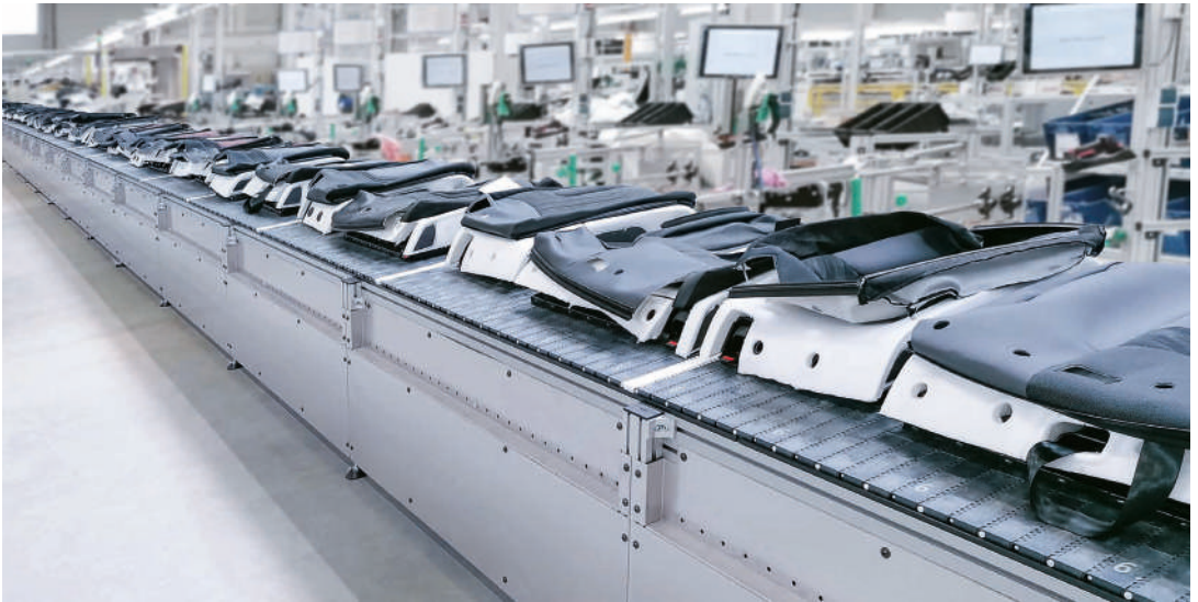
42 m long MBF-P 2040 with side creep zone protection and a protective guard for just-in-sequence mounting in non-stop operation
