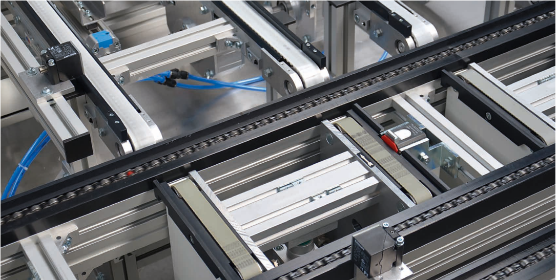
Separation of pallets from the main line in two parallel cross conveyor tracks
