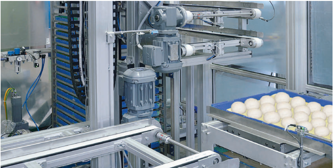
Interlink ZRF-P 2010 as loading and unloading station for bread roll production with stacking unit as a buffer
