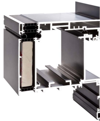
Thermally broken aluminium frame with 39mm polyamide thermal breaks and closed cell PIR insulation.
