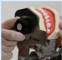
1) Attach the upper jaw model with the FE articulator to the headbase by tightening the upper fixing screw.
