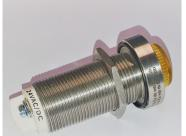
The JCE range of 'PL' explosion proof LED Pilot Lights are ATEX & IECEx certified, for fitting to control enclosures with compatible Ex d or Ex tb product certification. Suitable for industrial and hazardous areas, these pilot lights are of a robust design and offer good visibility under daylight conditions. They have an estimated life of 100,000 hours and an IP66 ingress protection rating.
