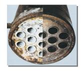
RYDLYME has been used for the effective cleaning of air compressors, boilers, chillers, condensers, cooling towers, and heat exchangers. The solution is easy to use as it is added directly to your equipment through fouled water passages and circulated by a portable pump.
