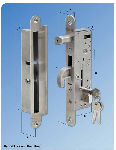
Ideal for folding sliding doors as it has an adjustable non-handed keep and a hook latch so that the doors cannot be folded if the flush bolts are unlocked. Another benefit is that the latch can be operated via the key so if preferred no handle on the folding side can be an option.
