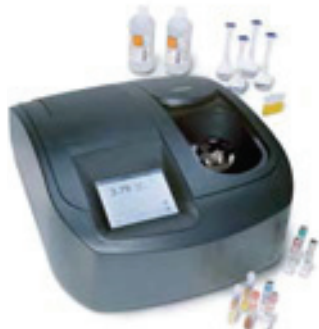
DR 5000 UV-VIS Spectrophotometer with high precision optics
