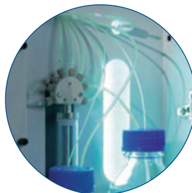
IL 500 TOC including autosampler with two-needle technology
