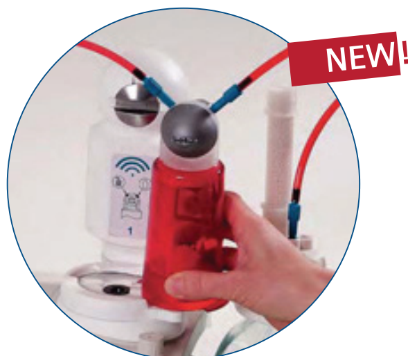
TITRALAB titration systems now with RFID—for simple and reliable GLP → See page 86
