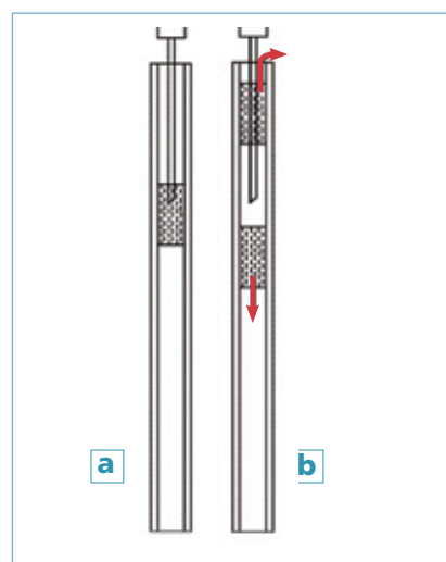
Figure 1. Conventional wool liner. (a) Wool plug is in the correct position to wipe needle tip (b) Wool plugs can be moved in either direction, preventing needle wiping
