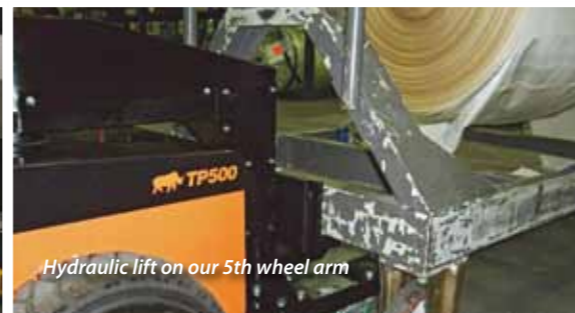
TP500 hydraulic with 5th wheel for moving 6,000 Kg train transformers.
