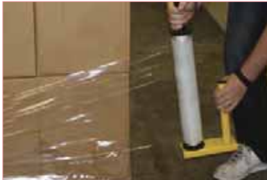
Economy dispenser for pallet stretch film W400-500mm x38/50/78mm cores
