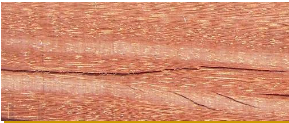
Typical fissures in Ekki
