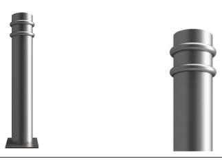
A substantial bollard with a clean appearance, the GFC6R Ornamental Bollard is constructed from mild steel and galvanised to ensure its longevity. Caps and rings of cast iron are welded on to the steel body to complete the design.
