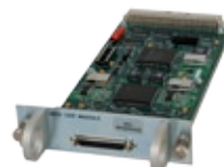
ECL CE 110MBPS MAX BITRATE 1BPS INCREMENTS ASYMMETRIC OPERATION
