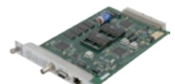
MANAGEMENT CARD MANAGEMENT VIA THE CONSOLE PORT, OR ETHERNET PORT USING SNMP OR TELNET
