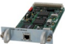
LAN CE 100MBPS WIRESPEED 1BPS INCREMENTS ASYMMETRIC OPERATION
