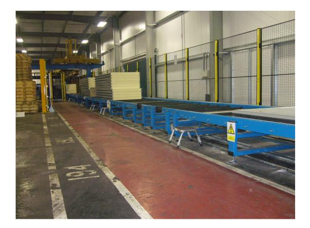
The SCM range of equipment includes heavy duty chain, roller & belt conveyor system, purpose built stacking / de-stacking systems, palletising units, pallet insertion units, in-line automatic wrapping machines, and robotic systems.
