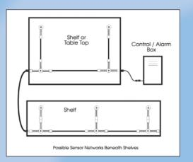
The sensors can be linked together into a variety of networks, and inserted beneath a shelf, panel, or other surface on which items are to be displayed. The sensors are inserted so as to fully support the weight of the display surface and the objects on it. The display surface can be of any stiff material, such as wood, glass, MDF, steel etc.
