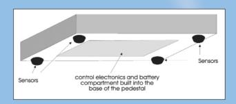
The maximum length of the alarm signal can be specified by the customer, and is factory set. The preferred duration can be adjusted by the operator up to the maximum time. On activation, the alarm will trigger for this length of time, and then reset automatically.
