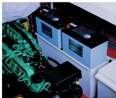
Installation of Lifeline batteries in progress on a Motor Yacht showing batteries being fitted into standard battery boxes.
