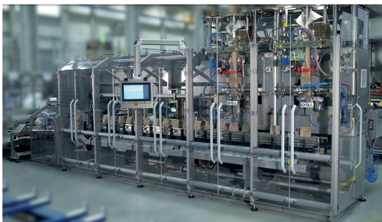
ROVEMA Block Packing System SBS TWIN: Flexibly adaptable to different bag shapes and packing materials. Up to 160 packs/min.
