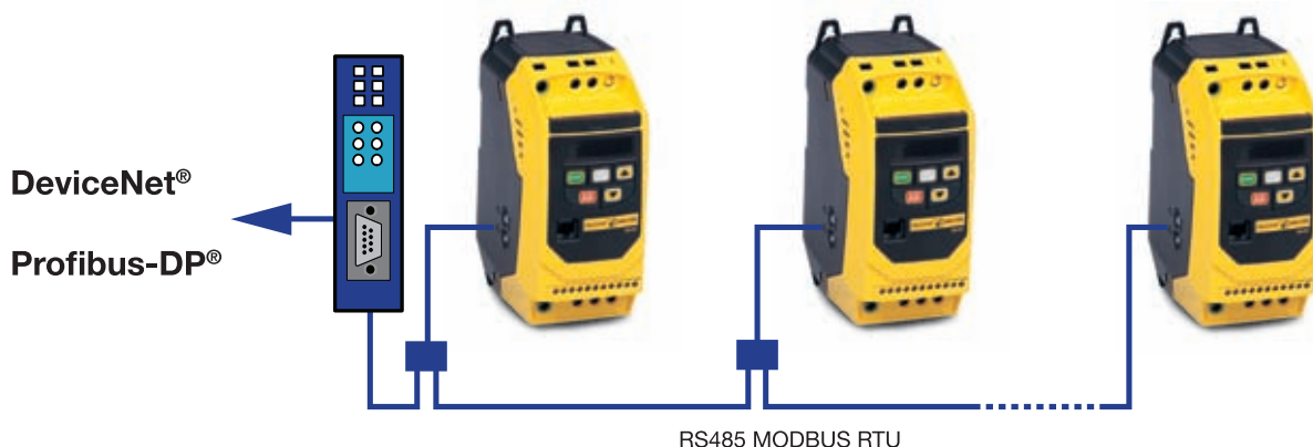
RS485 MODBUS RTU
