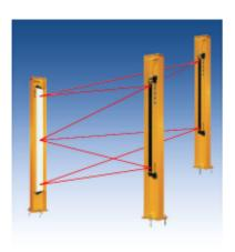
**FUTURA4/3R** is especially formatted for perimeter, zone or area protection. The three scanner beams within the optical device are in "cross matrix" array, which generate a total of nine beams of IR light. The beams are positioned equidistance in accordance with the requirements of European standard "EN999" for positioning as a perimeter guarding system.
