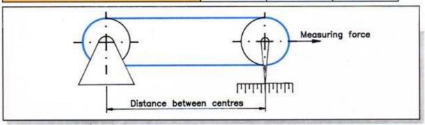
The effective length is verified placing the belt on two equal pulleys (diameter = 30 mm) having same groove profile.
