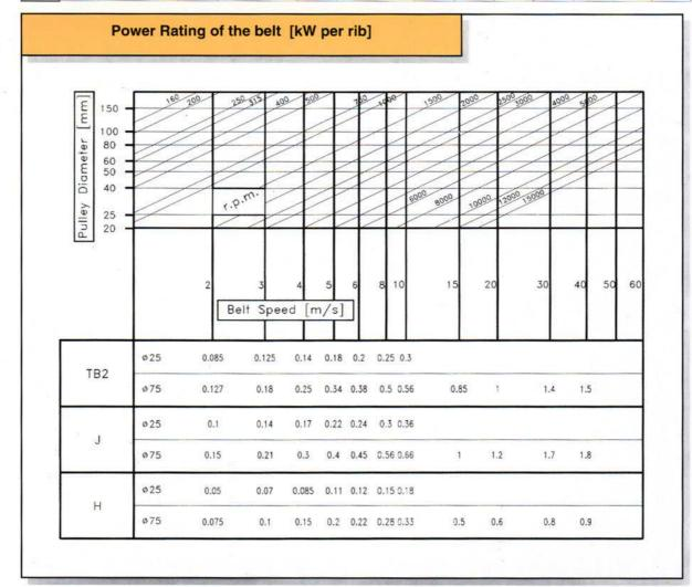
Recommanded installation tension per cm belt width for the endless form 300 N Length elongation with recommanded tension 0,7%
