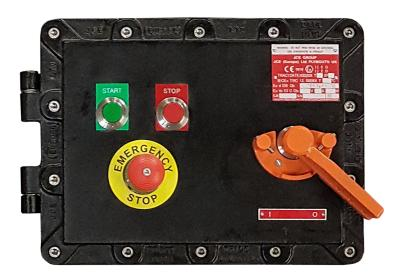
The JCE range of MSA/B/C Flameproof (Ex d) DOL Motor Starters are intended for use in areas made potentially hazardous by the presence of flammable liquids, gases or vapours (Zones 1, 2, 21 and Zone 22). Certified for Group IIB locations.
