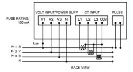
**CAUTION:** The instrument is suitable for connection to a 415VAC 4 wire STAR system. Connection is made via the terminals marked VOLTS INPUT. Phase 1 (RED) should be connected to V1, phase 2 (YELLOW) to V2 and phase 3 (BLUE) to V3. The Neutral (BLACK) cable is connected to the terminal marked N. For single phase systems voltage connections to V1 and Neutral only are required.
