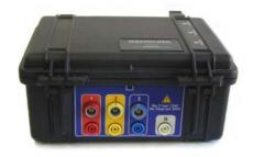
The measurement performance is equally impressive... the EnergyPro measures True RMS Voltage, Current, Power Factor and Energy with a high level of accuracy (+/-0.5%) and utilises a standard 32MB flash card for memory storage. Safety in use is given a high priority – voltage measurements can be taken from a standard wall socket even when measuring 3 phase supplies and the unit conforms to IEC 1010 Cat III 600V electrical safety standards.
