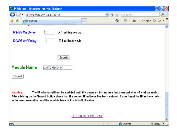
Module Name: This field allows you to enter a module description name into the Converter Module. This is an identifier for diagnostic/maintenance purposes and is chosen to best describe the Converter Module in the system by name or number.
