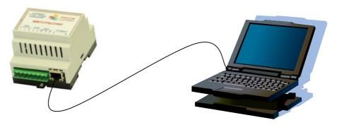
To setup your PC to connect directly to the Converter Module, an IP address in the same range as the Converter Module must be assigned to the PC. In Windows environments, this should be done as follows:
