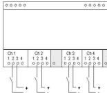
External DC power supply is connected between + and – as shown, in series with the output contacts.
