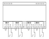
Terminals 1& 2 on each channel are looped as shown.
