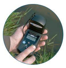
Once the light protection cap has been fitted, measurement can start: Simply press the button to read. The large display will show the result.
