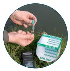
Out in the field: Samples are added directly for the pre-configured LANGE cuvette test. The cuvette is ready for use after a short development time.
