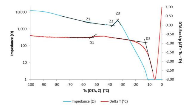
The Lyotherm analysis showed transitions both on the DTA and Impedance lines which have been summarised in the table below.
