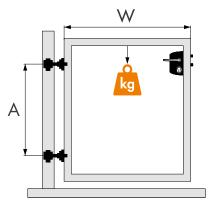
**SAFETY FACTOR 3,5**  $\frac{W}{\Delta} \leq 2$ A = Distance between the hinges W = Gate width
