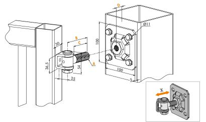
Vandal-proof one way 90° hinge with adjustable steel wall plate
