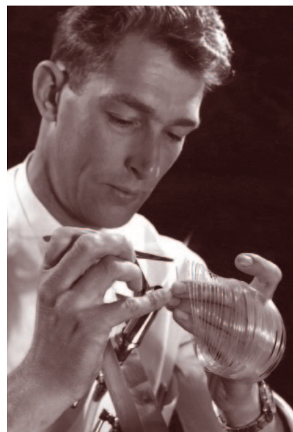
Founder Ern Dawes making an early glass GC capillary column, 1959.
