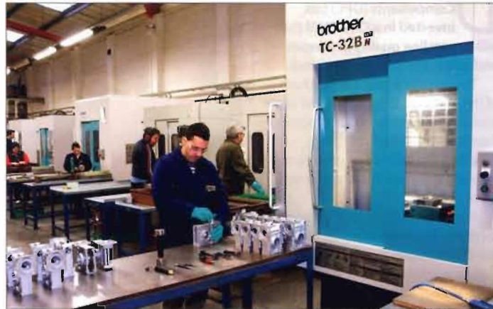
The six Brother high-speed machining centres in operation at RD Castings
