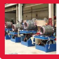
A generator manufacturing plant had a material handling issue as operators were required to work at fixed height benches. However, unless the operator was of average height there was the potential that they could suffer from a Repetitive Strain Injury or any other related bending and twisting type injury.
