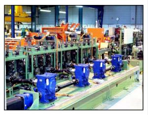
**F2(50)-16-DUPLEX SERVO ROLLFORMER** A 16 pass duplex servo rollform mill with 50mm diameter shafts. Variable speed low inertia servo drive, with drive transmitted to the forming heads via telescopic propshafts.
