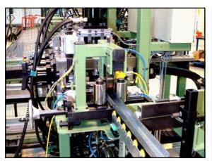
**TWIN HEADED INKJET PRINTER SYSTEM** Each print head will mark products coming from the rollformer with the required text. An encoder is mounted onto the strip to give the system a speed feedback for printing.
