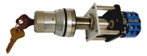
The JCE Group range of 'KS' explosion proof Key Switches are ATEX & IECEx certified, for fitting to control enclosures with compatible Exd product certification. Suitable for industrial and hazardous areas, these Key Switches are of a robust design and offer reliability during continuous operation. All devices are designed with IP66 ingress protection rating.
