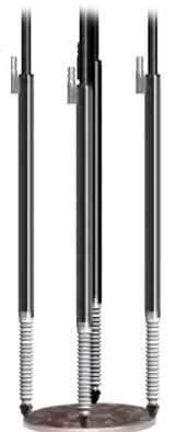
6 mm Probes Checking Flatness of a Coin
