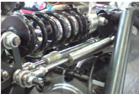
APPLICATION: S-SERIES TRANSDUCER MONITORING AUTO FRAME
