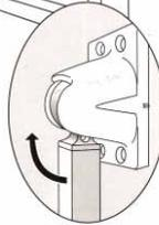
Slidelok Bar rotates up inside jamb
