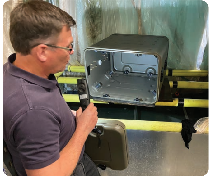
Internal inspection after water test
