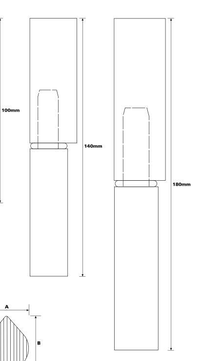
**Note: Ball bearing washer** increases overall height by 4mm approx. Ball bearing washers are recommended for heavy duty doors and doors which are in constant use. The bearing assembly consists of 2 hardened steel cones in a steel case.
