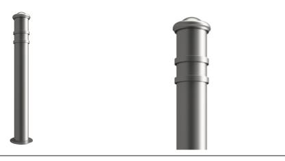
The GFC1700 Ornamental Mild Steel Bollard from AUTOPA is suitable for a wide range of locations and purposes. Constructed using mild steel, then galvanised to ensure its longevity. Cap and rings are welded onto the steel tube to complete the design.
