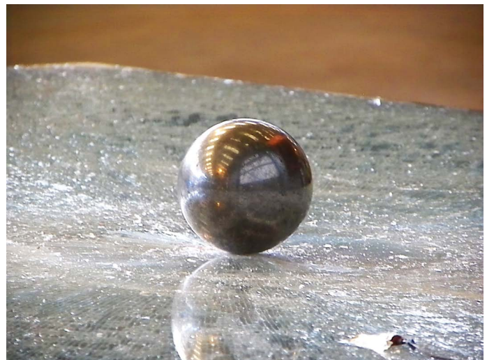
Steel ball used in hard body impact test.
