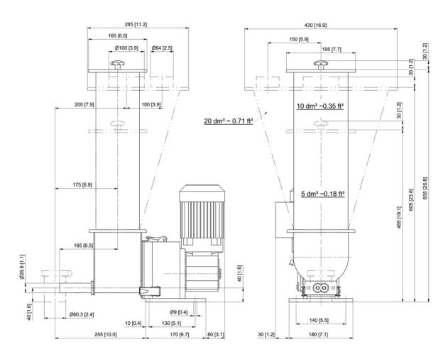
Weight without extension hopper approx. 16 kg (35 lb) Weight with 5 dm $^3$ /0.18 ft $^3$  extension hopper approx. 19 kg (42 lb) Weight with 10 dm $^3$ /0.35 ft $^3$  extension hopper approx. 21 kg (46 lb) Weight with 20 dm $^3$ /0.71 ft $^3$  extension hopper approx. 25 kg (55 lb)
