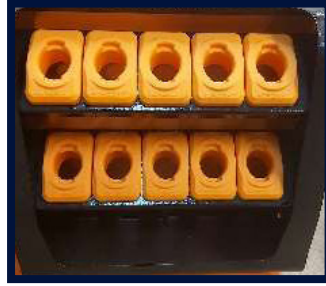
Integrated Holder for Tapping Bits
