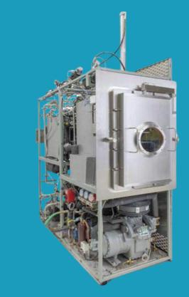
\* Hull LyoConstellation ™ S10 Aseptic Freeze Dryer as seen at the Biopharma Group GMP facility
